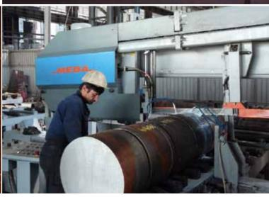
Annual production capacity is up to 80,000 tons of various qualities of steel ingots, such as: carbon steel, alloy steel, spring steel, chisel steel, die forging steel, high strength special steel, etc. Steel is supplied as ingots and the ingots are weighing up to 50 tons.
