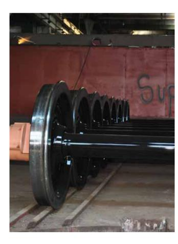
Welded or casted bogies are manufactured starting from semifinished laminates and castings or forgings which are machined and assembled to formsubassemblies components of the bogie (bogie frame, wheelhouses brake, suspension) which together with the running gears compose the complete bogie. During manufacture essential components are inspected and tested at various stages to certify functionality and reliability of the bogie.
